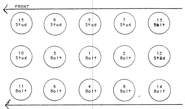
NOTE: Bolt & Stud No. Indicate the Torque sequence on tightening. You have 6 studs & 9 bolts, on the 134 Flat Head.
